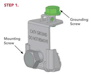
Back off both hex mounting and green grounding screws on connector to allow clearance to mount on front top lip of meter panel (left or right side).
