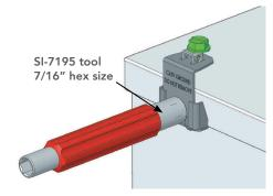
Use SI-7195 tool to firmly tighten hex mounting screw.
