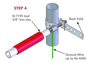
Release top set screw and insert up to a #6 AWG copper ground wire. Tighten set screw firmly to secure the ground wire using SI-7195 tool. Thread end of ground strap through slot of ground tag SI-TAG-100 and fold back any excess ground strap.
