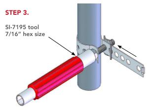
Slide S captive nut to align with set screw stud assembly. Tighten stud assembly firmly around pipe using SI-7195 tool.
