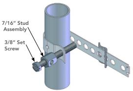
Wrap ground strap around pipe and align set screw stud assembly to match closest hole to pipe on opposite side of ground strap.
